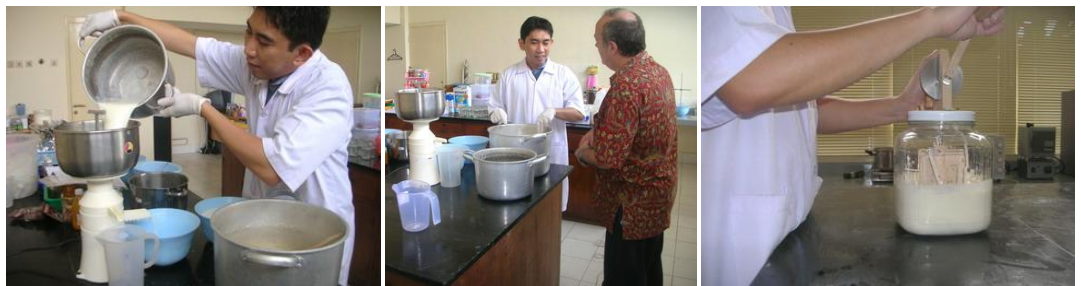
Left-right: Pouring raw milk to a cream separator machine, a brief discussion upon the process, converting milk cream to butter by using the manual butter churn
